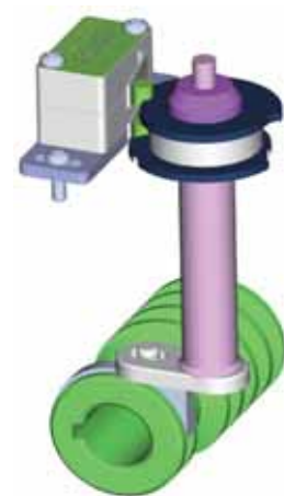
Fig.8: Mechanical limit of over torque
