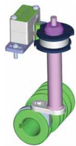
Fig.9: Mechanical limit of over torque
